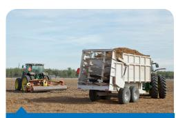
A modified spreader and a rototiller spread and incorporate chips from an entire orchard at a field demonstration that took place at Tallerico Farms in Manteca in October.
